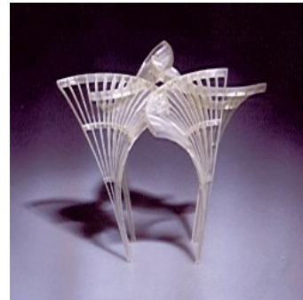
Figure 27: CALM project - final object produced by stereolithography (James Jackman). Reproduced by kind permission of the Learning Development Unit
