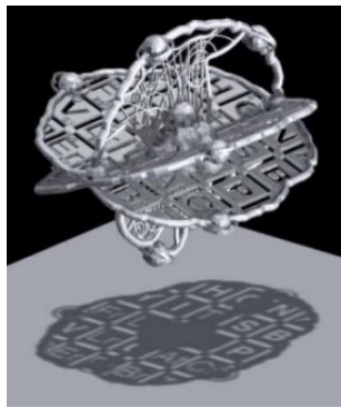
Figure 26: CALM project - 3D image and final object produced by fused deposition modelling (Justin Marshall). Reproduced by kind permission of the Learning Development Unit
