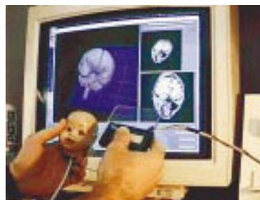
Figure 103: Environment for neurosurgical planning with “passive real-world props”. [Goble, Hinckley et al. 1995] Reproduced by kind permission of IEEE, © 1995 IEEE
