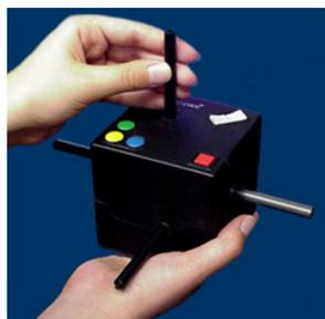
Figure 102: CubicMouse™. Image courtesy of Fakespace Systems Inc.
